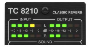
The LED meter section at the top of the hardware module gives feedback about the incoming and outgoing audio signals. The input level displays the audio as it enters the plug-in, and the level is not affected by adjustments to the input level control or any other parameter. The output meter is affected by the results of the effect, as well as the output level control parameter.
