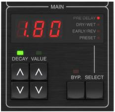
The numerical display in the Main section shows the current value of the DECAY, or the current parameters for PRE DELAY, DRY/WET, EARLY/REV, or the current Preset number.
