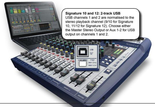
The Signature 10 and 12 consoles have 2-track USS input and output functionality. This could be used for recording a mix to a PC or Tablet, for example - or to use a computer as a playback device. Channels 1 and 2 are received by the highest-numbered stereo channel (9/10 for Signature 10, 11/12 for Signature 12).
