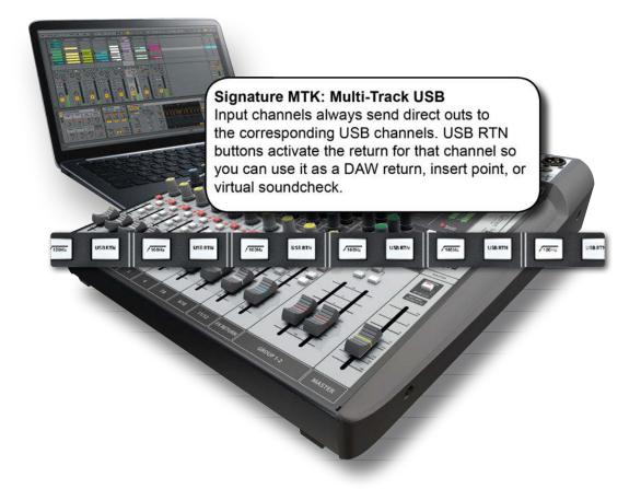
The Signature 12MTK console also has Multi-Track (MTK) output and input functionality that allows sending of direct outputs from the input channels and return USB audio channels directly to the input channels.
