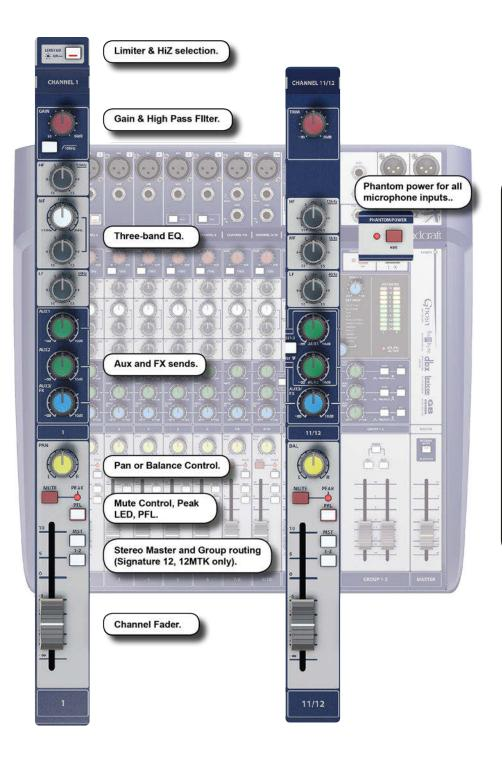
The controls are shown in the order they appear on the console channel strip - from top to bottom. This is not necessarily signal path order. Please refer to the relevant signal path diagram (section 4).
