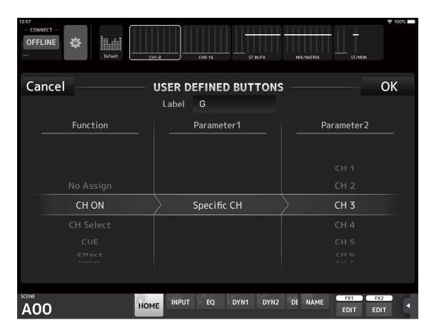
Tapping the text box for configuring Label enables label text to be entered directly via the keyboard. You can enter up to 6 characters. It can also be left blank.
