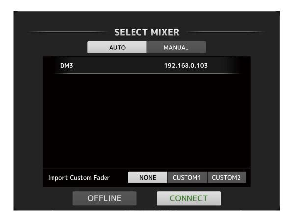
The Unit Name and IP Address of DM3 Series console found in the network are displayed in the list.
