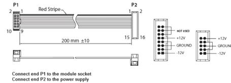
Connect end P1 to the module socket
