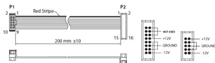
The unit comes with the required power cable for connecting to a standard Eurorack power supply system. Follow these steps to connect power to the module. It is easier to make these connections before the module has been mounted into a rack case.
