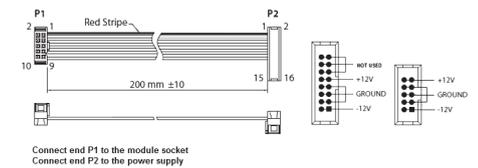
Connect end P1 to the module socket
